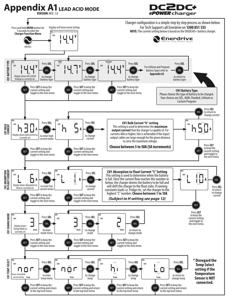
NOTE: At any function setting, pressing the MENU button will exit the function mode.
